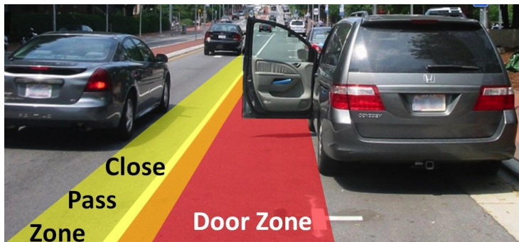
Figure 3 Avoiding the door zone
